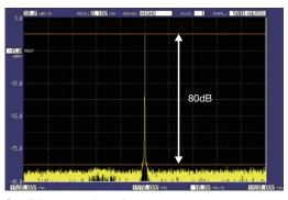
Straylight suppression ratio (high dynamic mode: = off, high performance model)
