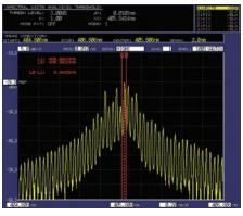
405 nm FP-LD measurement (resolution setting: 0.01 nm)
