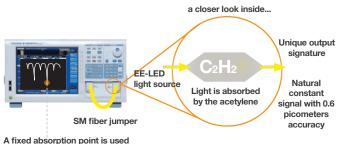
to re-adjust the internal calibration table
