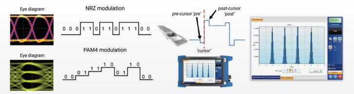
Pre-emphasis and RX equalizer tools help users adjust and manipulate the signal characteristics for TX (cursor and eye location) and RX (including different types of DSP modes) validating each lane of the pluggable under test. Once these parameters are modified, users need to identify the impact these parameters have over the PAM4 eye diagram. Our PAM4 histogram tool provides a detailed graphical view of each lane diagram directly on the screen of the tester, showing values for each PAM4 level.
